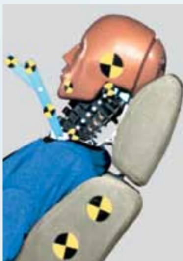
Good seat/head restraints start with good geometry. The restraints are positioned high and close behind the head.
