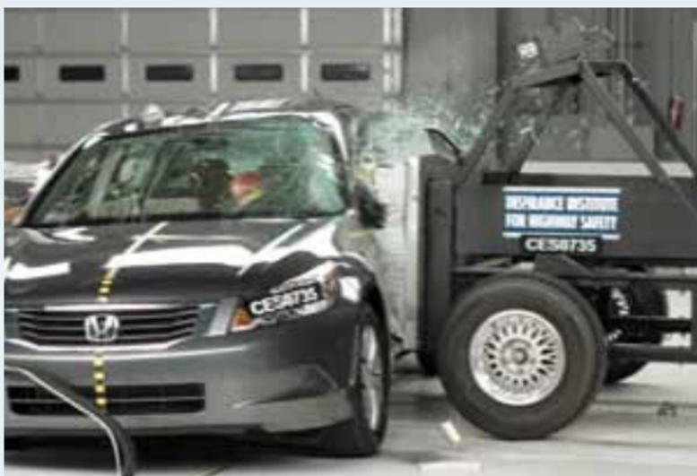
In the Insurance Institute for Highway Safety's side crash test, the striking barrier is higher than in the federal government's test, so it mimics crashes in which occupants' heads are at risk. Choose a vehicle that earns a good rating in this test.
